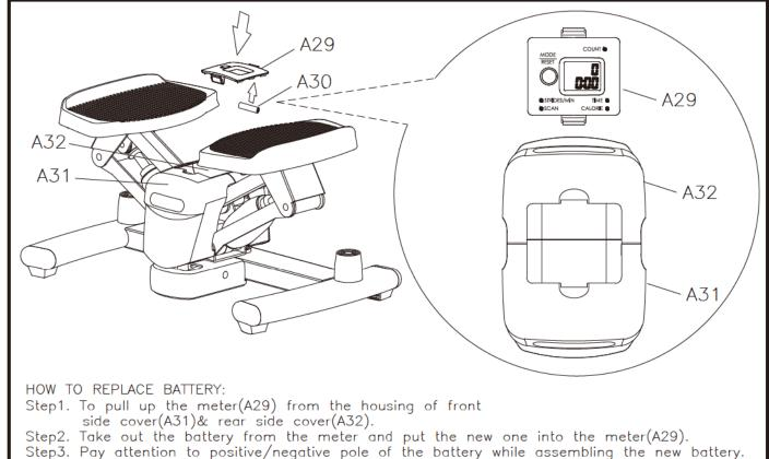
Step3. Pay attention to positive/negative pole of the battery while assembling the new batte Step4. Equip the meter(A29) onto the housing of front side cover(A31)& rear cover(A32).
